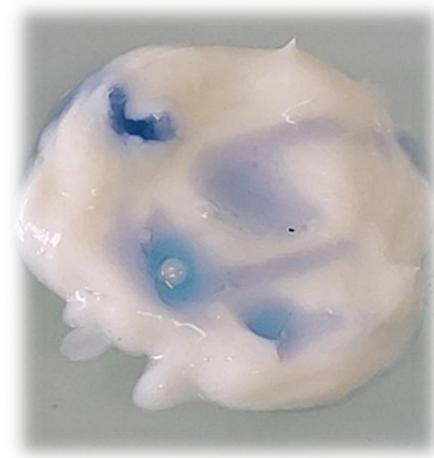
**Fig. 6.** Colorimetric reaction of methylene blue on the antifungal emulsion formulated with *Pistacia lentiscus* L. vegetable oil.
