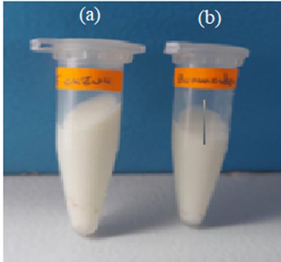
**Fig. 5.** Stability of emulsion after centrifugation (2000rpm for 15 min) with *Pistacia lentiscus* L. vegetable oil from the two regions of Algeria (Tizi Ouzou (a) and Boumerdes (b)).
