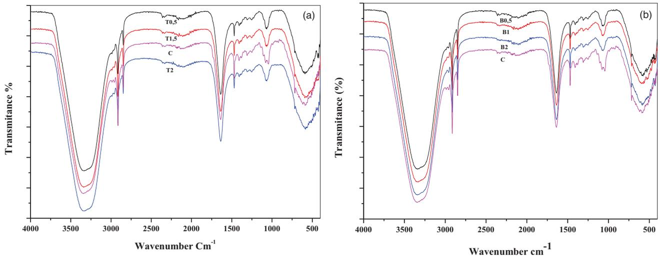
**Fig. 8.** IRTF spectra of control antifungal emulsions and these prepared with *Pistacia lentiscus* vegetable oil from two Algerian regions : (a) IRTF spectra of Tizi Ouzou lentisk oil (b) Boumerdes lentisk oil. Boumerdes emulsion 0.5, 1.5 and 2 g of lentiscus oil (B1, B2 and B3), Tizi Ouzou emulsion 0.5, 1.5 and 2 g of lentiscus oil (T1, T2 and T3) and Phanazol reference (c).
